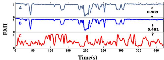
**Figure 2. Repeated recordings of identical screen content lead to nearly equivalent EMI traces (Panels A vs. B, Lion King, correlation = .989), while content from different movies produce distinct electrical noise patterns (B vs. C; Lion King vs. Bourne Ultimatum, correlation = .402).**
