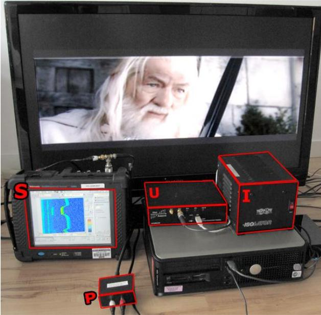
**Figure 3. Recording Hardware Setup.** S = Spectrum Analyzer, P = Power Line Interface (PLI), U = Universal Software Radio (USR), I = Isolating Transformer. The Sharp 42" LCD TV and the data logging PC are also visible.
