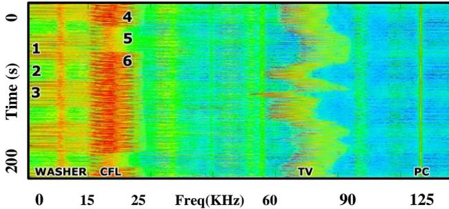
**Figure 1: Frequency domain Waterfall plot of the EMI spectrum in a home (red = high amplitude signal, blue = low amplitude). Note the dynamic nature of the TV EMI from 60 KHz (dark scene/low power consumption) to 90 KHz (bright scene/high power consumption). Interesting events for other devices are labeled numerically**
