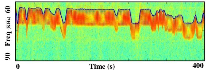
**Figure 4. Raw FFT signal around the EMI band of the TV. The result of post-processing this signal to extract the EMI trace features is overlaid as the blue time series. Note that unlike Figure 1 which also shows raw FFT data, the time axis is now along the horizontal.**
