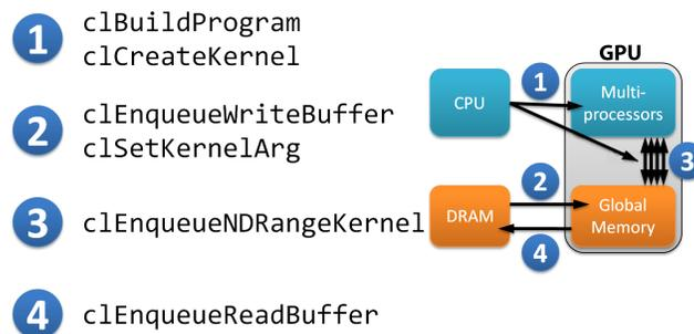
[Figure 2]. Essential aspects of the OpenCL workflow.
