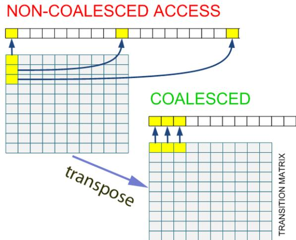
[Figure 7] Transposing the transition matrix to coalesce memory accesses.
