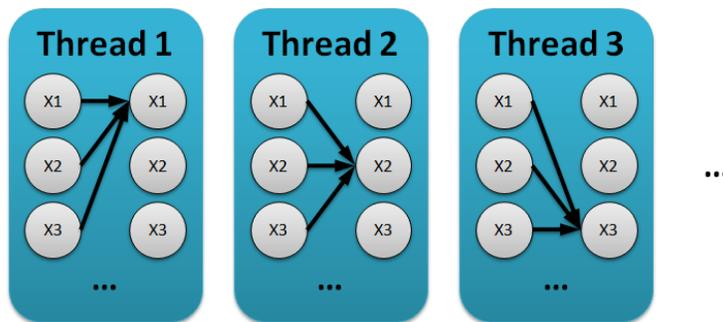
[Figure 5] The  $i$ -th thread is responsible for updating the probability of state  $i$  (at time  $t$ ).
