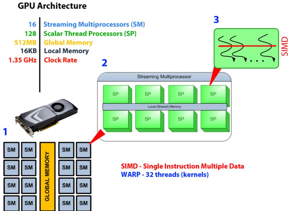
[Figure 1]. The GPU architecture is broken down into three levels of detail. At the highest level is a set of 16 streaming multiprocessors (SM) with shared access to 512MB of global memory. Each SM is composed of 8 scalar thread processors (SP) which are the core computational units. The SPs run synchronized warps of 32 threads which follow the single instruction multiple data (SIMD) paradigm. For additional hardware details refer to the Appendix.
